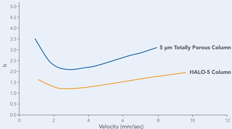
This comparison of van Deemter plots for HALO-5 and a totally porous 5 micron particle demonstrates the extraordinary low reduced plate height that is obtained from HALO-5 columns. The unusually narrow particle size distribution of the HALO-5 Fused-Core particles facilitate the packing of columns with efficiencies (theoretical plates) that are significantly larger than what would be expected from the size of the particles.
