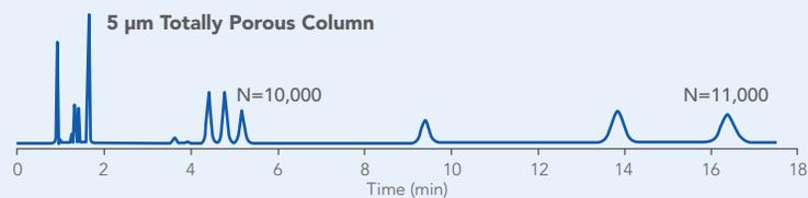
HALO-5 column separates this mixture of NSAIDs in less than 60% of the time and with better resolution than a typical HPLC column packed with totally porous 5 micron particles.
