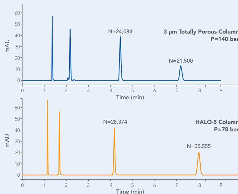
HALO-5 columns generate over 17% more plates than an HPLC column of the same dimension packed with 3 µm totally porous particles, but generates less than 60% of the back pressure.
