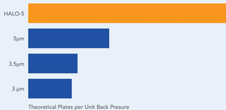
Columns packed with larger size particles will deliver more efficiency per unit of column back pressure. HALO-5 columns have a plates per pressure ratio that is significantly higher than what is seen with other columns packed with the same size totally porous particles. This characteristic of HALO-5 columns can be very useful when faced with developing a separation of a very complex mixture, especially when using HPLC equipment with limited pressure capability.
