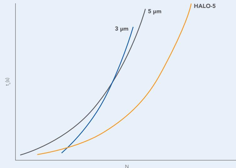
Kinetics plots are used to compare columns packed with different particles and particle sizes. This Kinetic plot compares columns of various lengths packed with HALO-5, 5 micron totally porous and 3 micron totally porous particles and shows that HALO-5 columns provide more column plates (N) for a given analysis time ( $t_r$ ) than columns packed with totally porous 5 and 3 micron particles.
